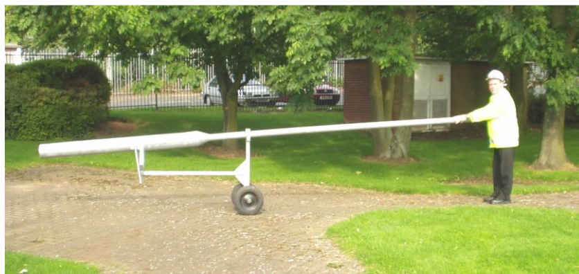
Figure 10-2 - Carrier and column ready for moving
