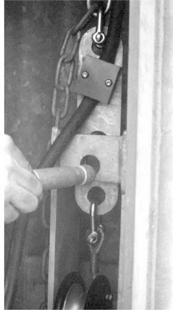
Fig. B – Remove pin from anchor plate
