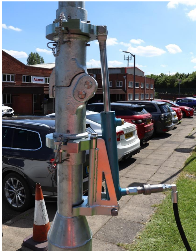
Figure 3 Lower and upper clamps situated on hinge body. Please note that the retaining pins on clamps may vary.
