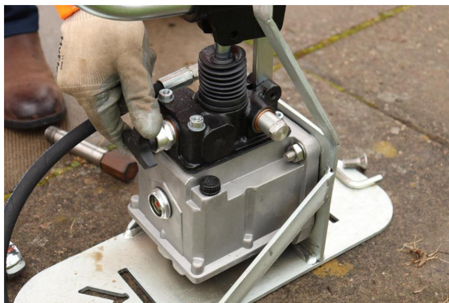
Figure 9 Adjusting pump unit pressure
